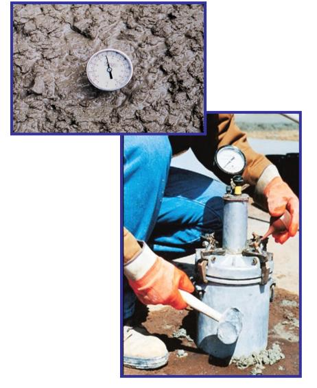
Less air is entrained as the concrete temperature increases.
