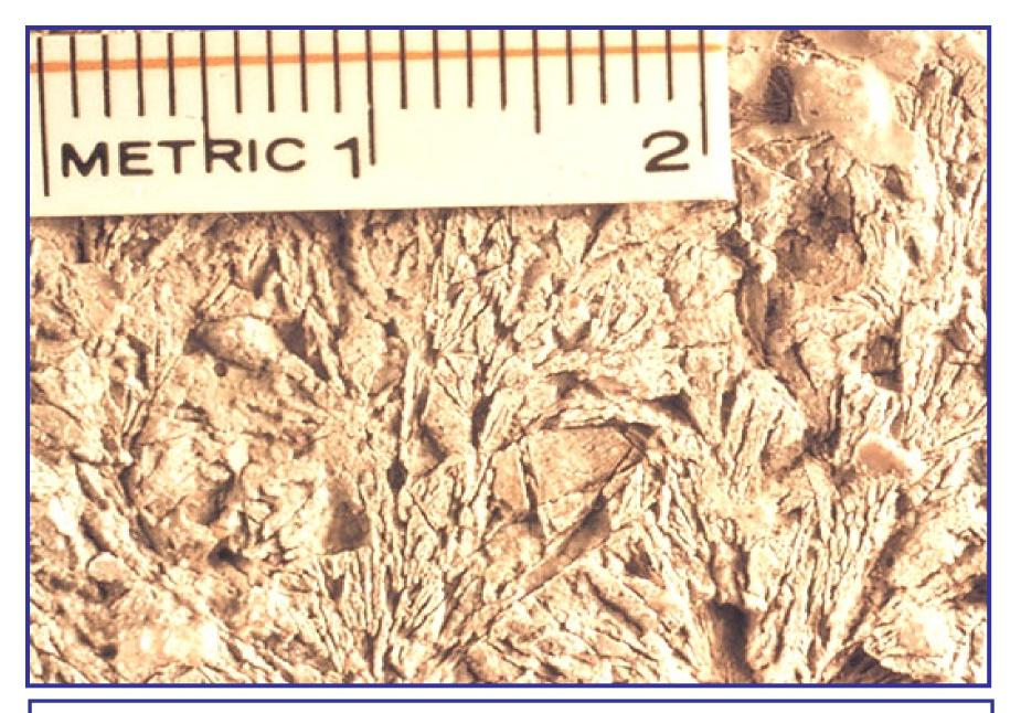
If batch water freezes,up to 50% strength reduction can occur<sub>7-22</sub>
