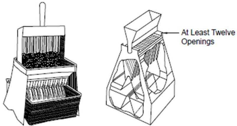
(b) Small Sample Splitters for Fine Aggregate
