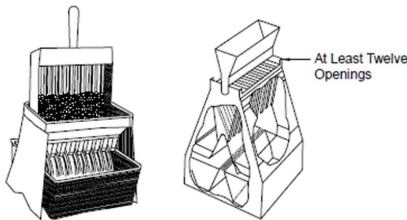
(b) Small Sample Splitters for Fine Aggregate
