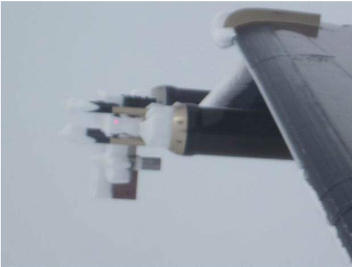
Fig 2: Icing on the instruments and CIP laser is blocked by ice (red spot) during middle of the flight around 2130 UTC.
