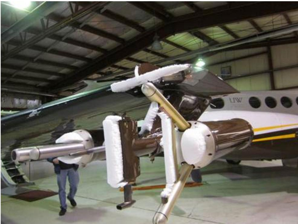
Fig 1: 2DP and FSSP pictures taken before (upper panel) and after (lower panel) the flight. Instruments are covered by ice during the flight.
