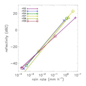
Numerical definitions of the equations are shown in the table below with **a** designating the prefactor, **b** the exponent, **c** the correlation coefficient, and **rmin** and **rmax** define the range of values for the data of given flight.
