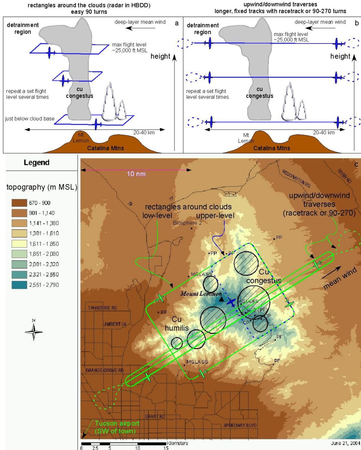
**Fig 2.** Modification of the environment by detraining cumuli. (a) box pattern, in clockwise direction to allow WCR coverage; (b) upwind/downwind traverses; (c) map display of (a) and (b).
