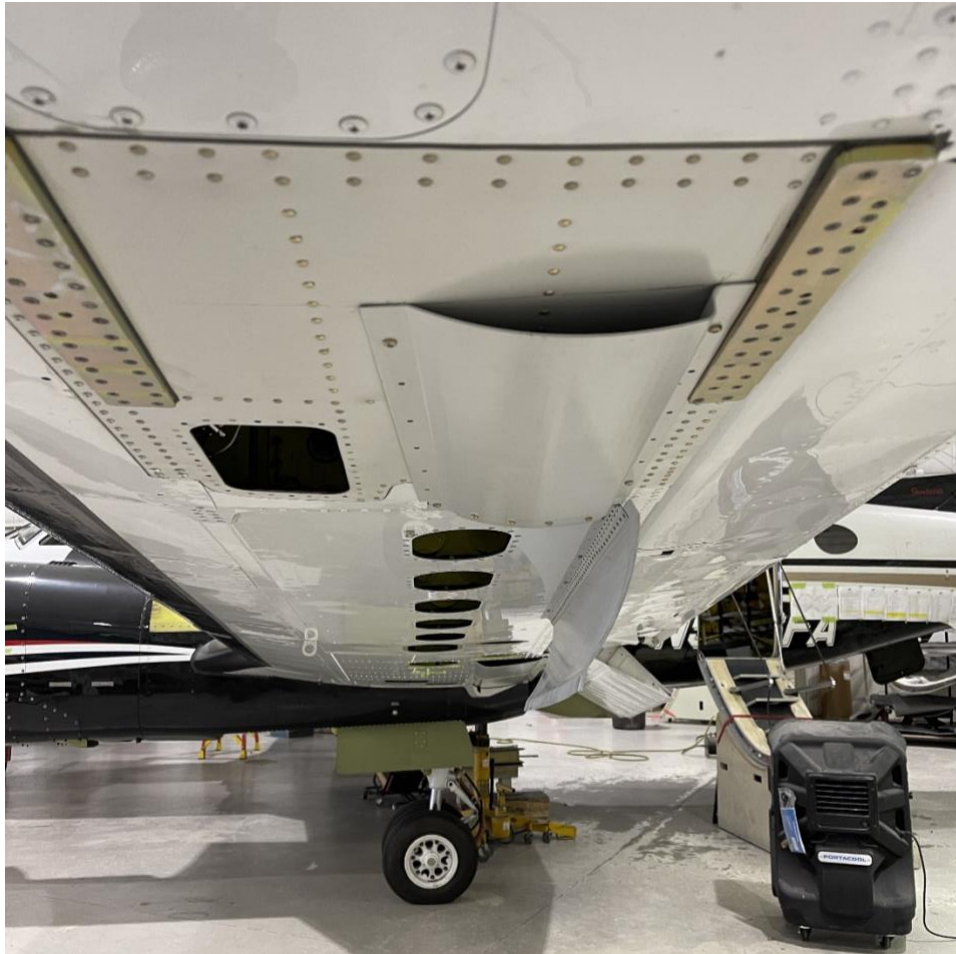
Figure 3.2.6 Wing External Electrical Conduits and Hardpoints (gold strips near top of photo)
