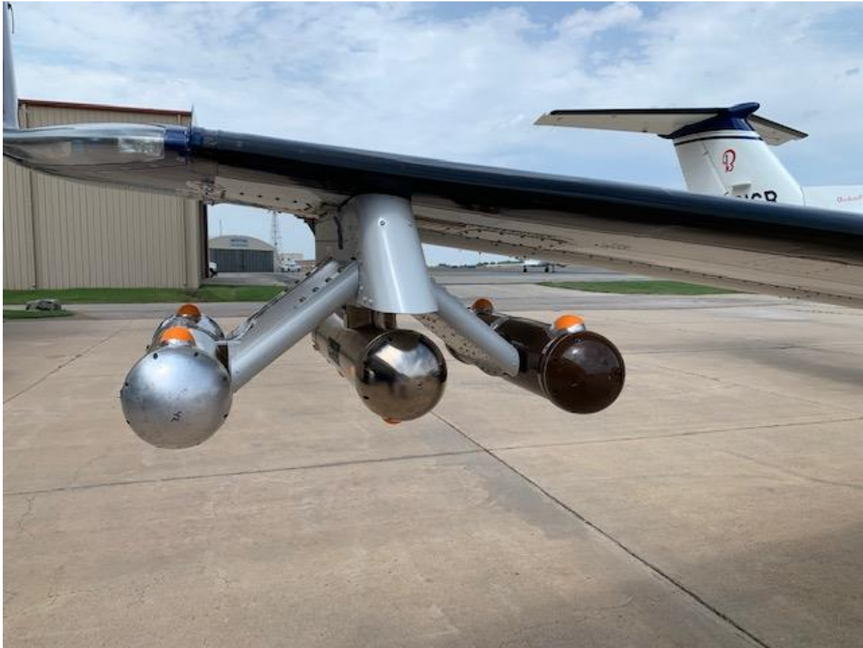
Figure 3.2.7 Wing Pylon and Research Canister Configuration Ready for Flight Test
