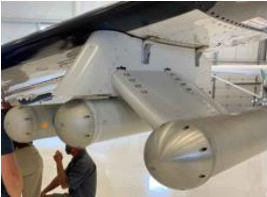
Figure 3.2.8 UW-provided “PMS” Instrument Canisters and pylon on FL-862
