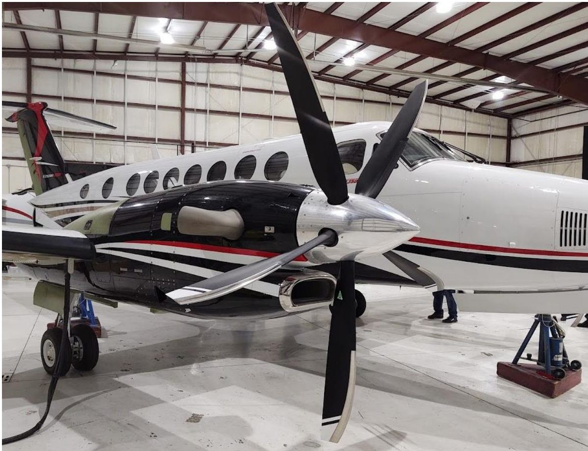
Figure 3.2.2 PT6a-67 engine with 5-blade composite propeller and heavy weight gear
