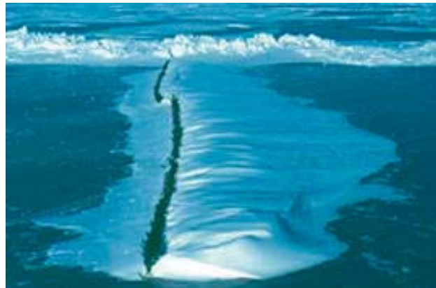
Photo 3. The research model shows how end effect reduces snow storage and increases wind velocity at the ends of the barrier.
