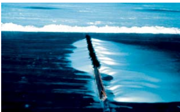
Photo 1. Research models show that density has a large impact on how a barrier will function. Note the drifting pattern created in the research model replicating the effects of a dense planting of trees in the upper barrier versus the effects a wooden snow fence would have (lower barrier).
