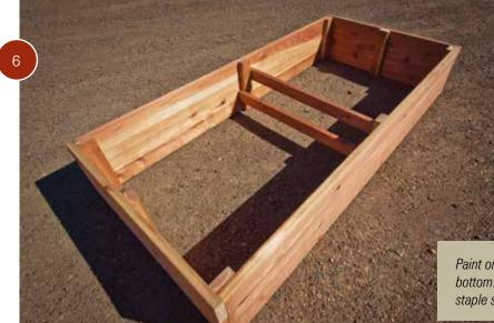
Paint on two even coats of wood finish (don't forget to finish the bottom!). Optional for trellis - trim wire fencing to 3'9"x7'9.5" and staple securely into place.
