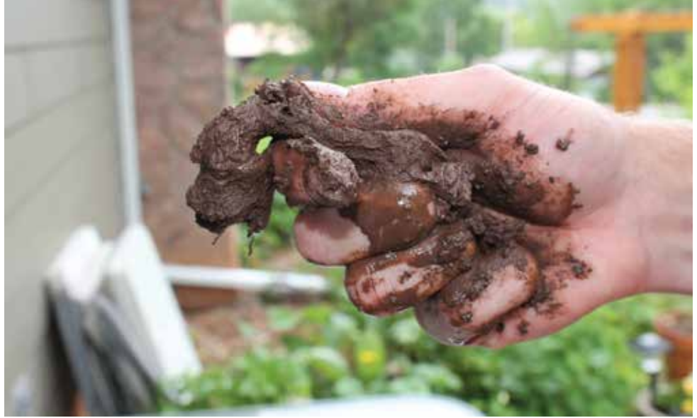
Hand texturing, while not as accurate as other tests, can be a reliable method.
