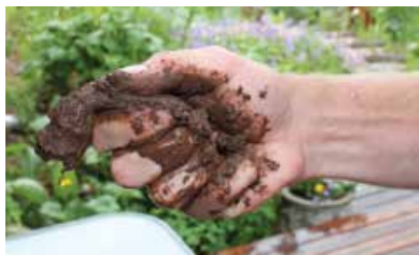
Begin squeezing soil between thumb and forefinger to make a ribbon.
