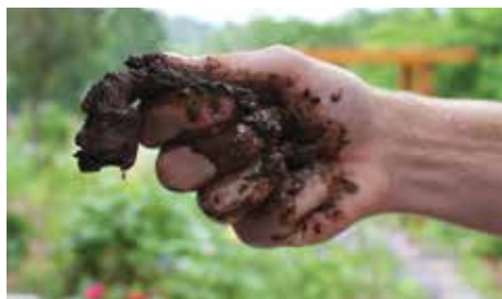
The length of the ribbon before breaking and grittiness of the soil determines the soil texture.
