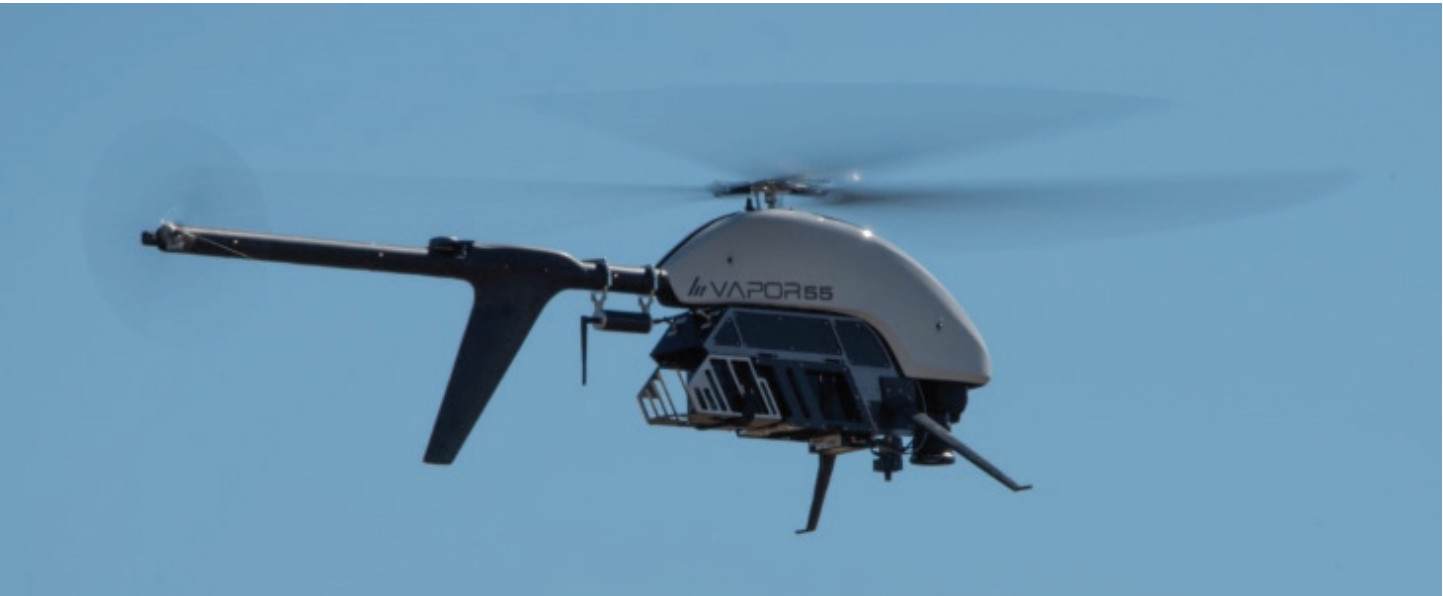
The Vapor 55 weighs in at a hefty 55 pounds and can cruise for about an hour.
