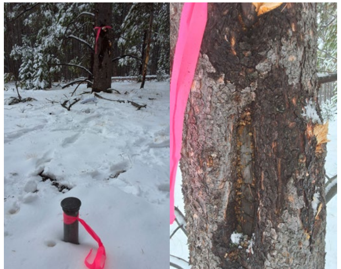
Figure 4. Official monuments recovered on Shirley Mountain. An iron post with brass cap monument and an accessory bearing tree, ca. 1966. Photos courtesy of the BLM.
