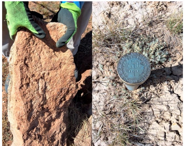
Figure 3. Official monuments recovered in Shirley Basin. Sandstone quarter section corner, ca. 1871, and iron post with brass cap section corner on range line, ca. 1938. Photos courtesy of the BLM.
