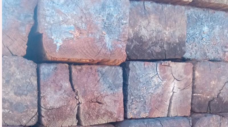
Railroad ties are not recommended for use in planters as they contain materials categorized by the EPA as probable human carcinogens.
