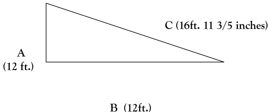
*Squaring the building is critical so that the rest of the structure proceeds normally in construction.*
