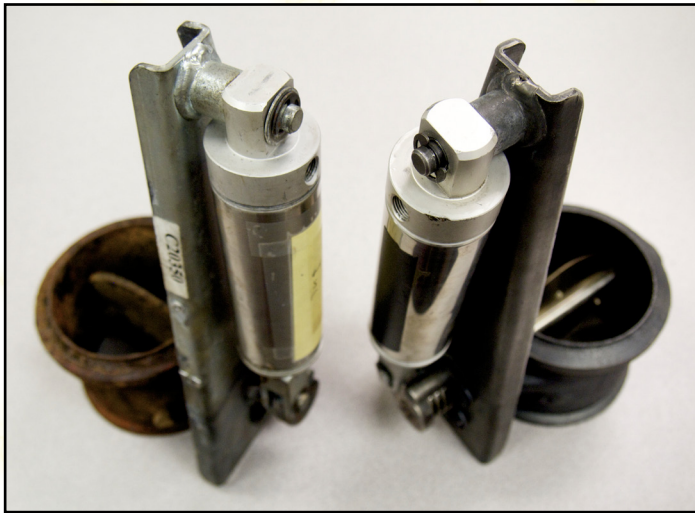
Original Exhaust Brake Design Improved Exhaust Brake Design
