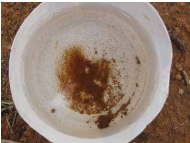
Soil sample that has disintegrated after swirling it
