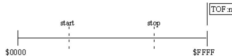
c) Case 3: Stop time count > Start time count, n timer overflows
