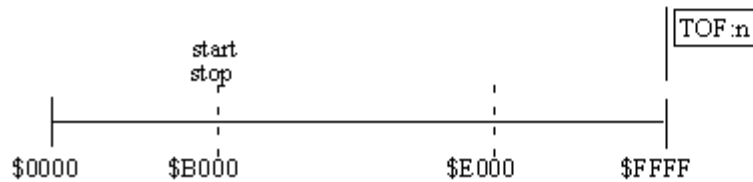
e) Case 5: Start time count = Stop time count, n timer overflows
