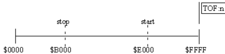
d) Case 4: Start time count > Stop time count, n timer overflows
