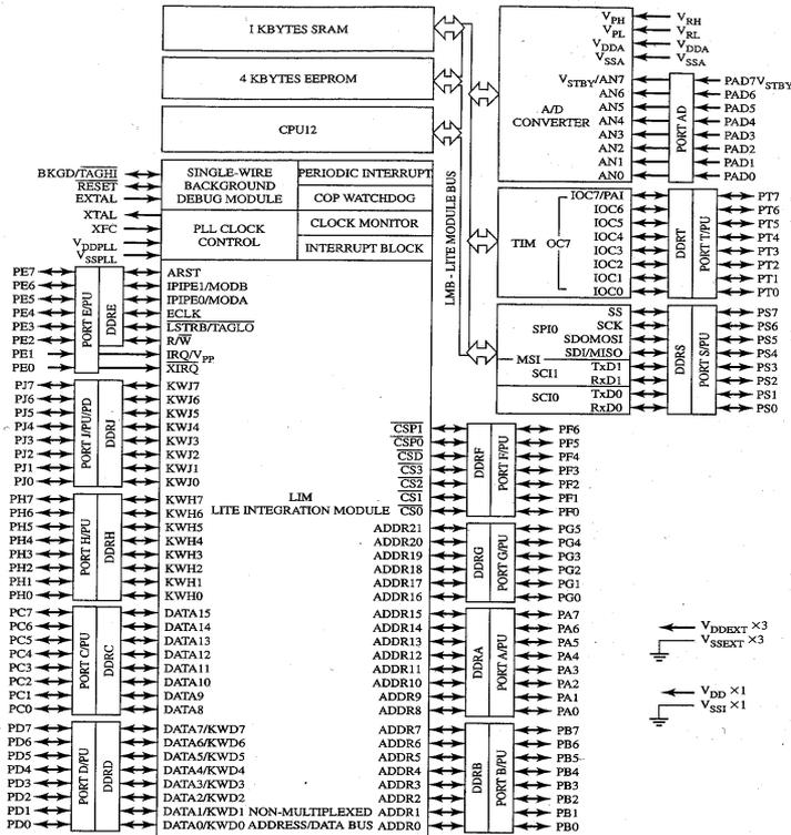
Figure 1.3 The block diagram of the MC68HC812A4 (Motorola).
