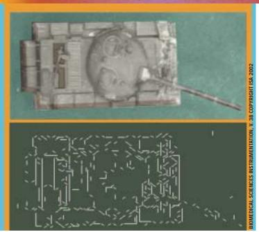
Digital processing demonstrates edge-recognition of a Soviet tank model. Edge recognition is a key to the success of missile tracking technology being developed by researchers at UW and the U.S. Air Force Academy.
