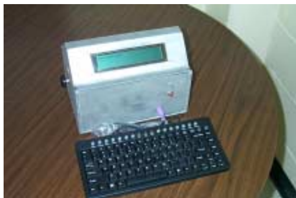
Figure 1. Personal Communications Device for Individuals with Speech Impairments.
