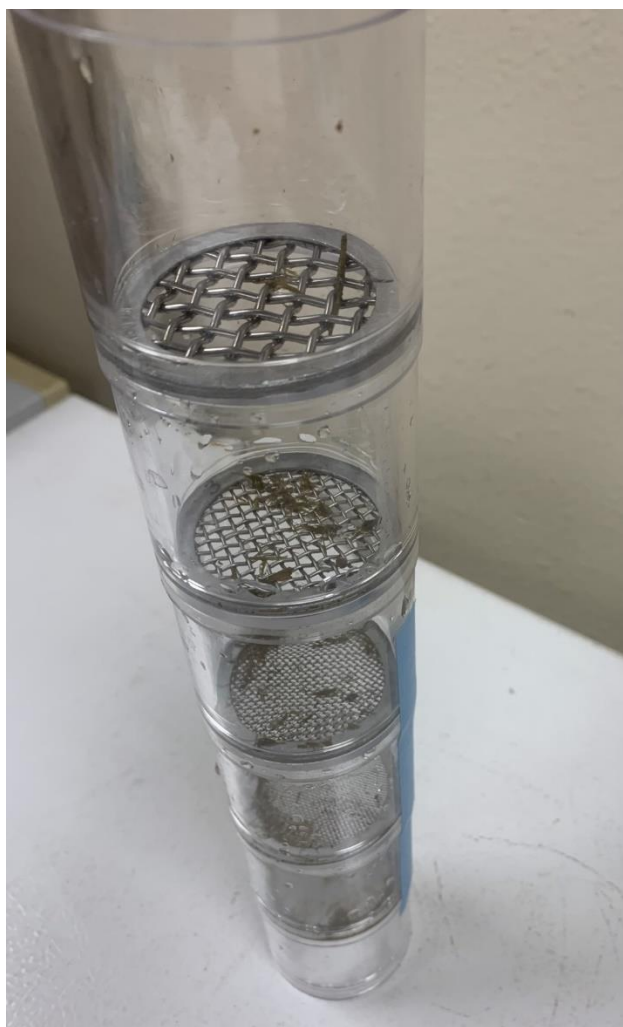
Figure A2: Example of a completed sieve stack using the traditional method after rinsing and before removing the metal sieves to be dried.
