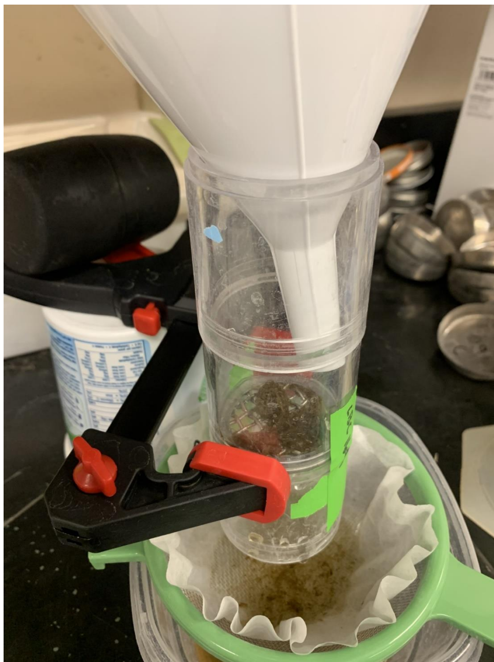
Figure A4: View of the simplified method after a sample has been run through the set-up and before rinsing.
