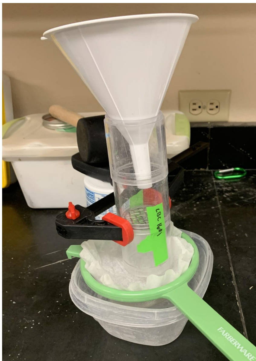
Figure A3: View of the setup of the simplified method before a sample is run through the sieve set-up.
