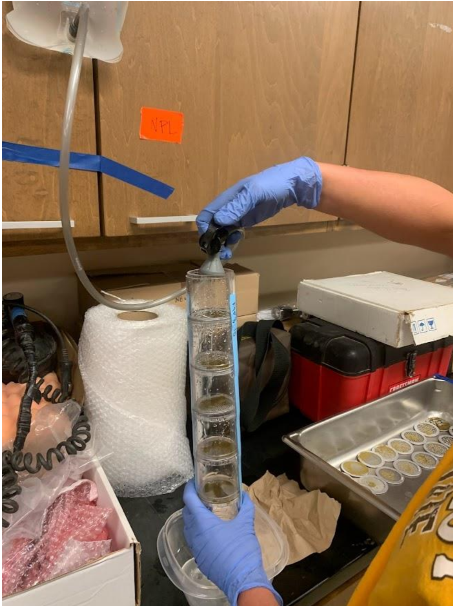
Figure A1: View of the sieve set up during the rinsing phase of the traditional method.
