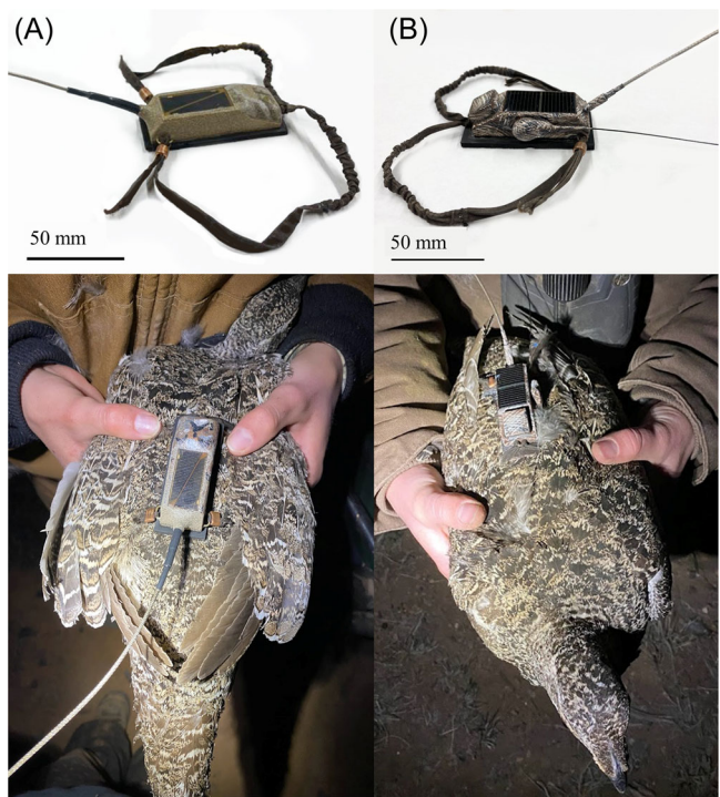
FIGURE 1 Two commonly used solar powered GPS-Argos satellite transmitters made by Microwave Telemetry, Inc. (A) and GeoTrak Inc. (B) with each company's individual transmitter in the photos located above photos of their deployment on greater sage-grouse ( Centrocercus urophasianus ) in Utah and Wyoming between 2011 and 2019 (photo credit: C. Backen).
