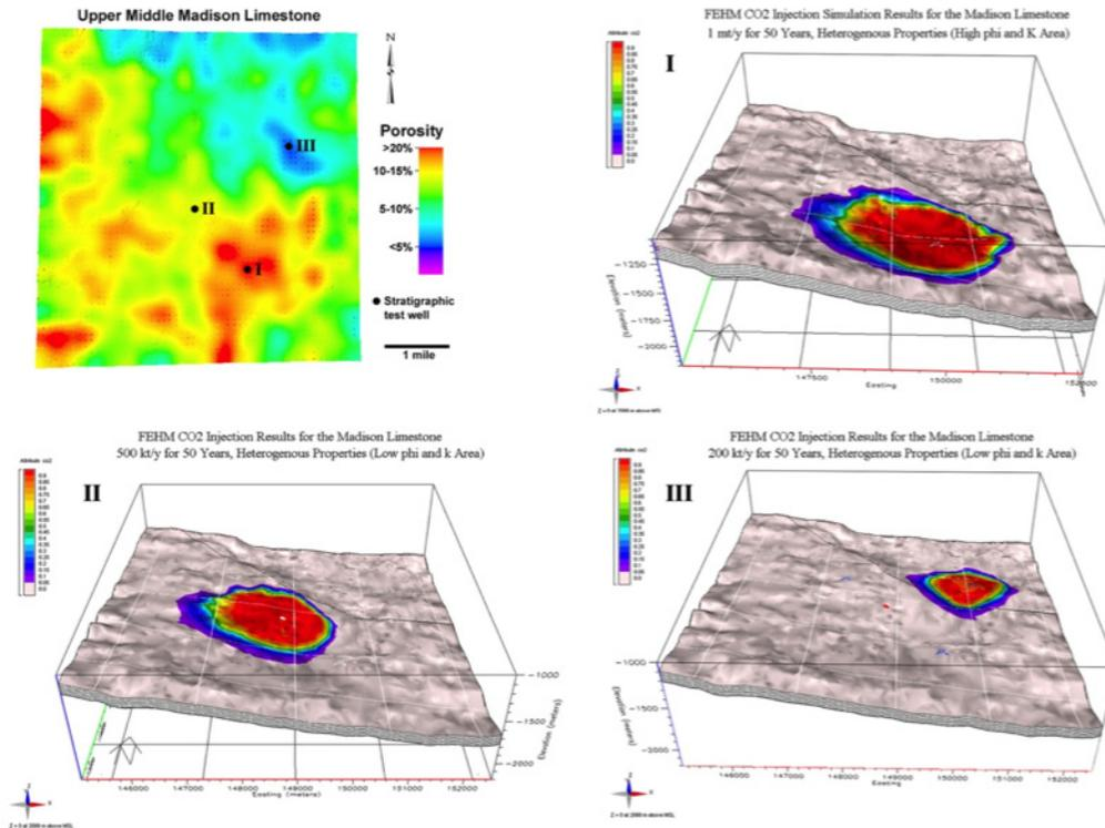
**Figure 9.** Diagram showing the size of the CO<sub>2</sub> plume resulting from CO<sub>2</sub> injection into the Madison Limestone from CO<sub>2</sub> injection at three locations in the study area (shown in upper left panel).
