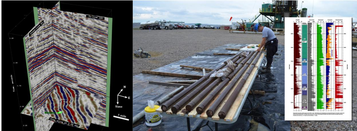
**Figure 2.** From left to right, this figure shows results from the 3-D seismic survey, core from the stratigraphic test well, and a well log suite from the WY-CUSP study site at the Rock Springs Uplift.
