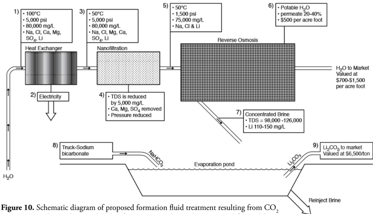
**Figure 10.** Schematic diagram of proposed formation fluid treatment resulting from CO<sub>2</sub> injection into the Madison and Weber formations on the Rock Springs Uplift. Potable water and metals are produced from the fluid, and residual brines are reinjected.
