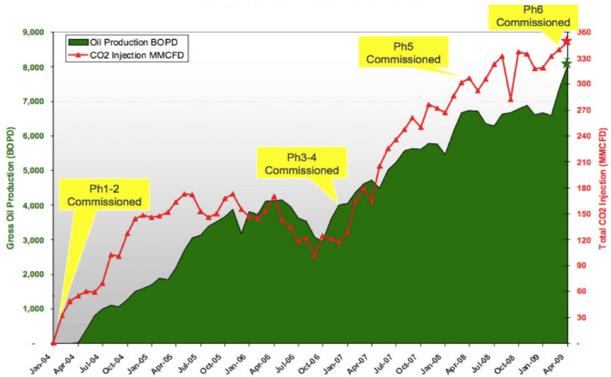
Figure 12. Example of CO<sub>2</sub> flooding and stranded oil recovery at the Salt Creek Oil Field.
