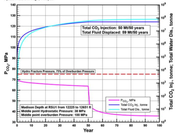
**Figure 8.** Output from numerical simulations of two CO<sub>2</sub> injection scenarios. The left panel shows a scenario in which only a small amount of formation fluid is produced during CO<sub>2</sub> injection, while the right panel shows a scenario in which the volume of formation fluid produced equals the volume of CO<sub>2</sub> injected (1:1 ratio). Note that in the left panel, CO<sub>2</sub> injection causes the pressure to rapidly approach fracture pressure.
