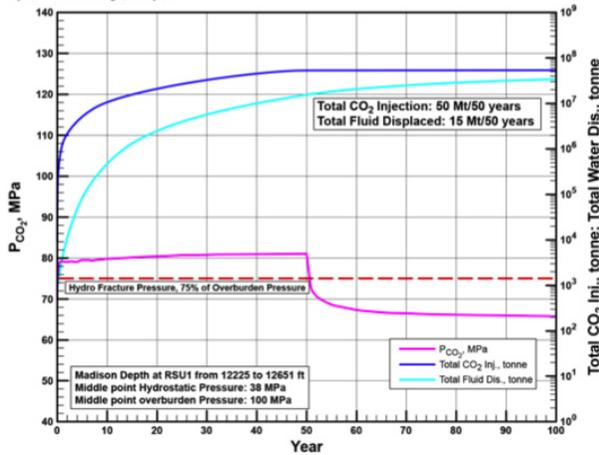
CO<sub>2</sub> Injection Simulation Results from FEHM for the Madison Limestone, Rock Springs Uplift
