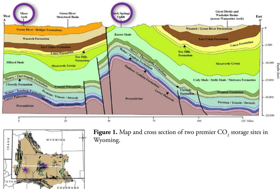
**Figure 1.** Map and cross section of two premier CO<sub>2</sub> storage sites in Wyoming.
