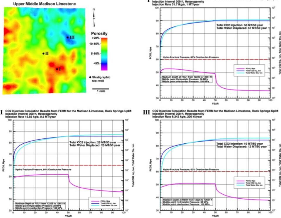
**Figure 4.** Numerical simulations of three CO<sub>2</sub> injection scenarios representing three different locations within the best reservoir interval in the Madison Limestone: the Upper Middle Madison.
