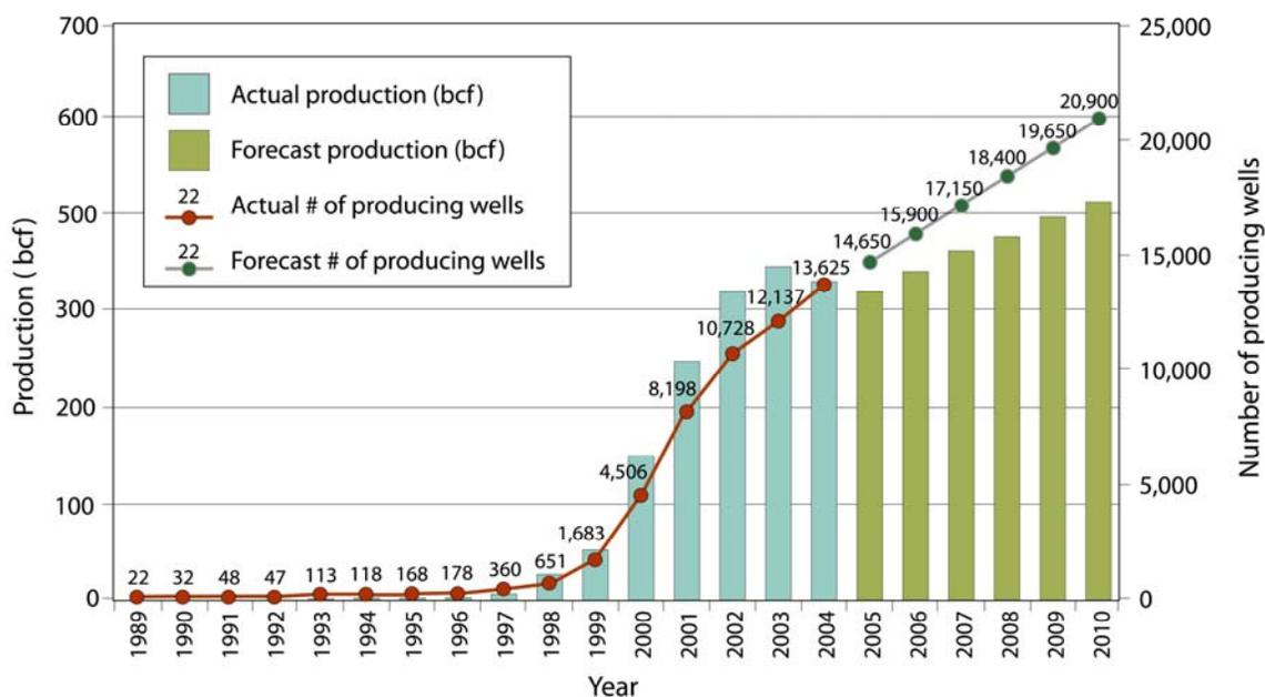
**Figure 1.** Yearly production and numbers of producing wells for coalbed methane in the Powder River Coal Field, Wyoming, 1989 through 2004, with forecasts to 2010 (modified from De Bruin, 2005). bcf = billion cubic feet.
