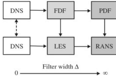
Figure 5.1.5: An illustration of unified turbulence models. Equations for filtered variables are given below. They can be applied as DNS-, LES- or RANS-models, depending on the choice of  $\Delta$ . The upper line shows corresponding stochastic models (SGS fluctuations vanish for  $\Delta \rightarrow 0$  such that FDF-methods reduce to DNS).
