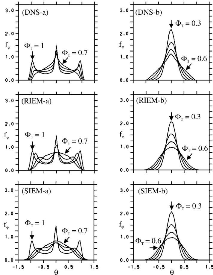
Figure 5.1.3: The evolution of a scalar PDF  $f_\varphi(\theta)$  as function of the progress variable  $\Phi_T$  which runs from unity to zero in time. The DNS data of Juneja and Pope [21] are given in (DNS-a) and (DNS-b), and the corresponding prognoses of the new mixing model in (RIEM-a) and (RIEM-b). The Figs. (SIEM-a) and (SIEM-b) show the performance of a simplified version of the new model.
