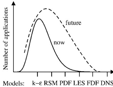
Figure 5.1.4: A slightly extended prognosis of Pope [3], who considered the current and future (next 10–20 years) use of turbulence models for industrial applications. RANS-models are split into algebraic ( $k$ - $\epsilon$ ) and Reynolds stress models (RSM) which apply transport equations to calculate Reynolds stresses.
