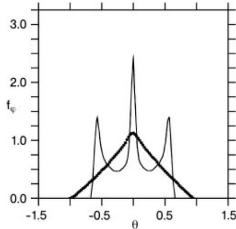
Figure 5.1.2: The dots present DNS data of the PDF  $f_\varphi(\theta)$  of a passive scalar (for  $\Phi_T=0.6$ , see Fig. 5.1.3). The thin solid line shows the corresponding predictions of the IEM-model for the evolution of the scalar PDF at this stage.
