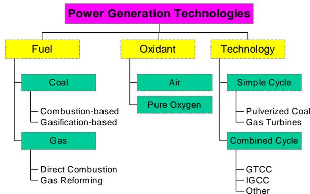
Figure 2. Technology Options for Fossil-Fuel based Power Generation
