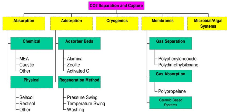
Figure 1. Technology Options for CO<sub>2</sub> Separation and Capture
