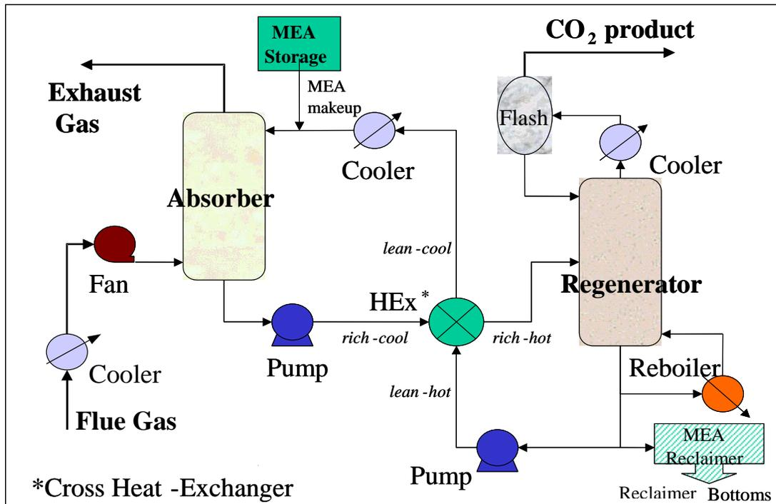
Figure 5. Flow Sheet for CO<sub>2</sub> Capture from Flue Gases using Amine-based System
