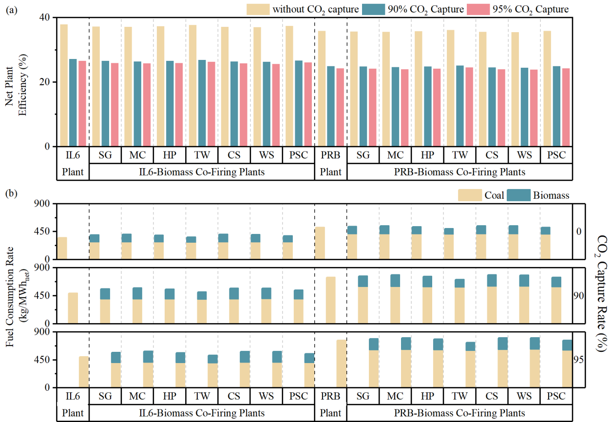
Figure 4.1. Performance of 20% Co-Firing Power Plants without and with CCS: (a) Net Plant Efficiency, and (b) Fuel Consumption Rate.
