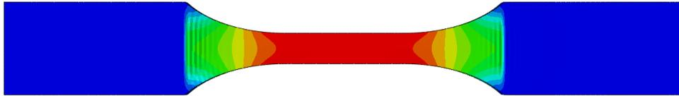
**Figure 2: Micro-tensile specimen stress distribution from finite element model**
