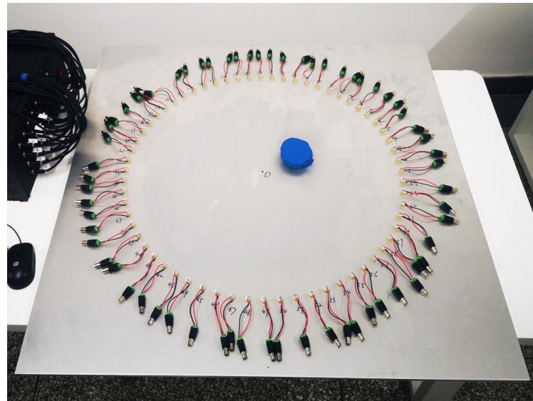
Figure 13. An aluminum plate with a piece of plasticine and 64 piezoelectric sensors.
