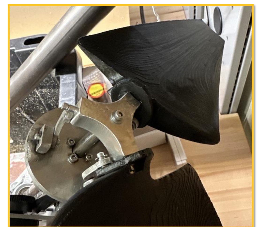
The initial broken blade and pitch system
