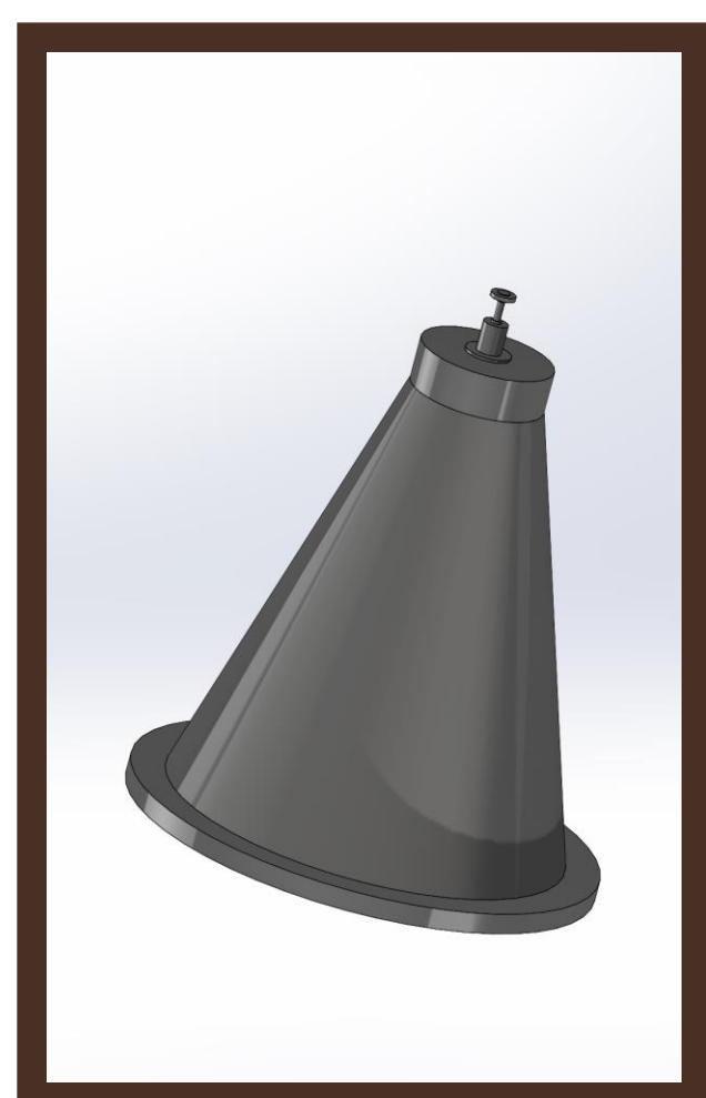
Pictured Right: Conical horn antenna, which is to be mounted on the zenith and zenith slant port.
