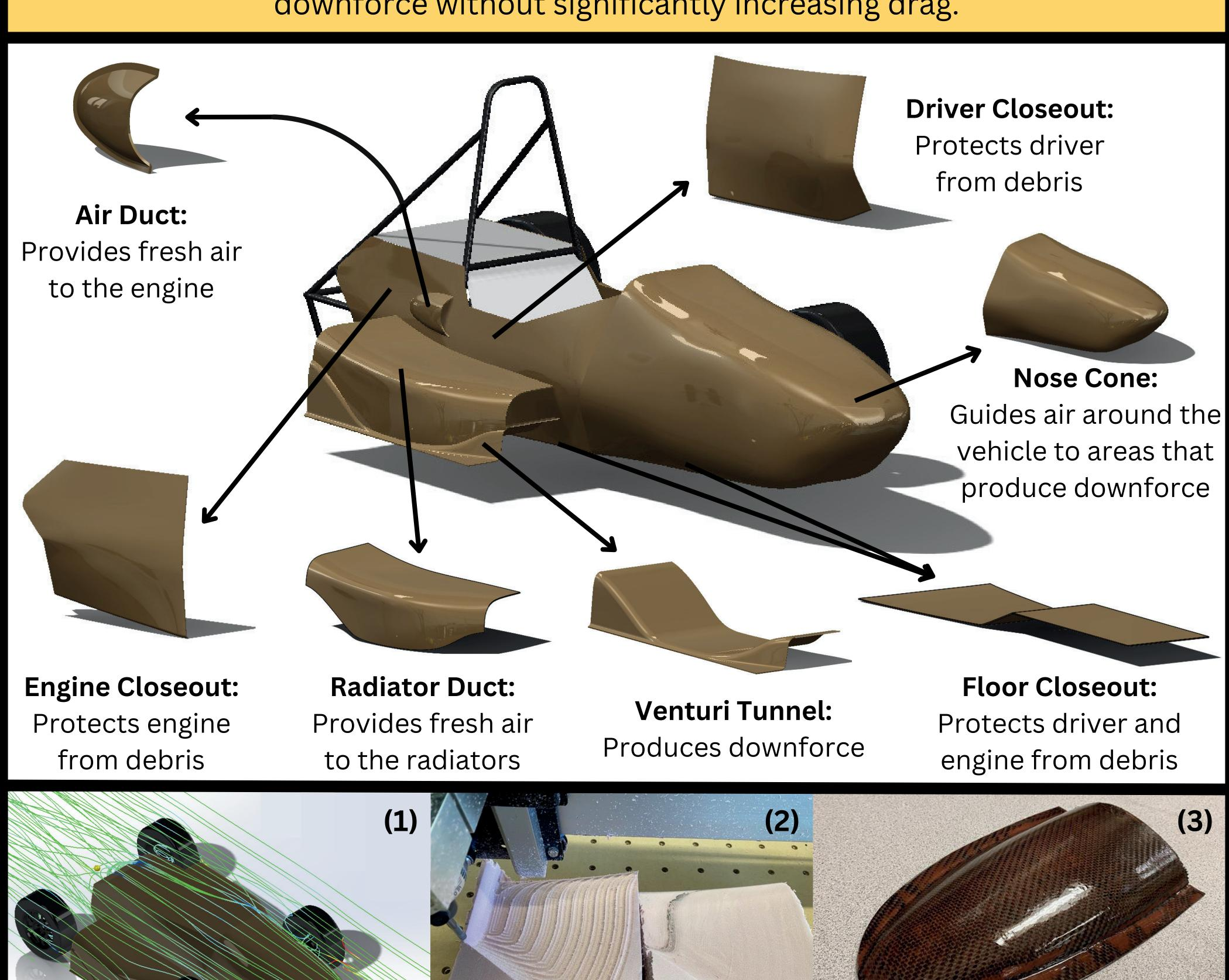
A model was developed and iteratively refined to optimize downforce (1). The most efficient version was converted to machine code to create molds for the layup process (2). Layups were performed on all components to fabricate parts, which were then post-processed and attached to the vehicle (3).
