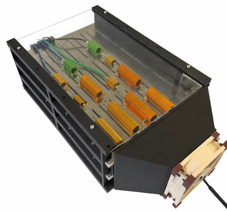
Figure 2: Load resistors and heat sink
