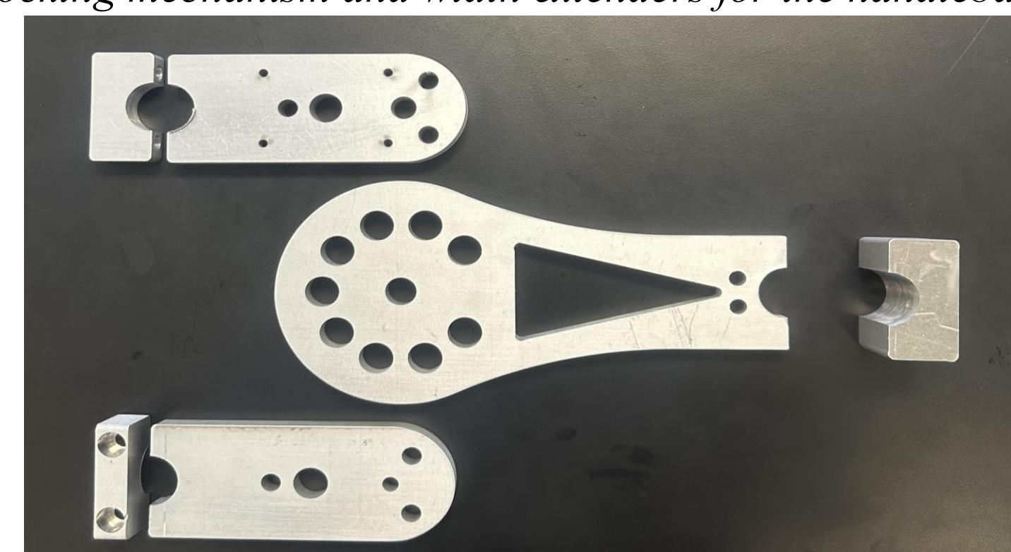
Figure 4: Manufactured pieces of the pitch joint to include the center section with locking positions and side pieces with standoff and pivot holes.
