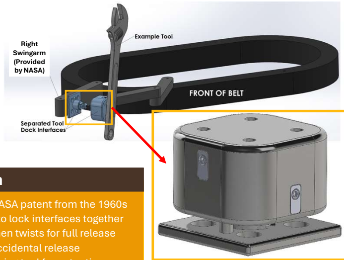
Pictured above: Mock-up view of NASA tool belt and swingarm system (top), full tool dock assembly (bottom)
