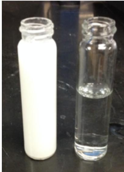
**Figure 15:** Images of the raw MF feed and its filtrate. The raw MF feed had a turbidity of  $>800$  NTU, while that for the filtrate was  $= 0.15$ NTU.
