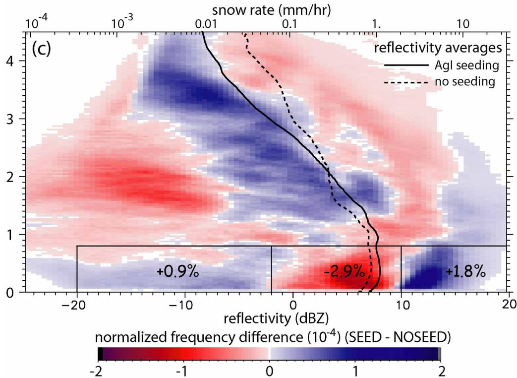
**Fig. 2:** Normalized frequency by altitude (FAD) of the difference in WCR reflectivity during seed and no-seed conditions. Also shown are cumulative normalized frequency differences (seed minus no-seed) in three boxes near the ground, expressed as a percentage, and the mean reflectivity profile during seed and no-seed conditions. The snow rate ( $S$ ) shown in the upper abscissa is inferred from  $S=0.11 Z^{1.25}$  (Matrosov 2007).
