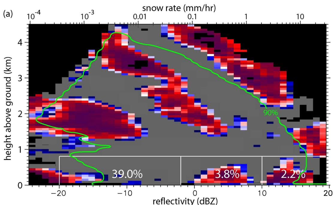
**Fig. 3:** Percentage of differences between randomly selected subgroups that exceeds the observed seed minus no-seed difference in WCR reflectivity (shown in Fig. 2). The white numbers show the same, not at the bin level but within the same boxes as in Fig. 2. In the grey areas there is a more than 10% probability that the seed minus no-seed difference is by chance. The green contour comprises 90% of the cumulative data frequency.
