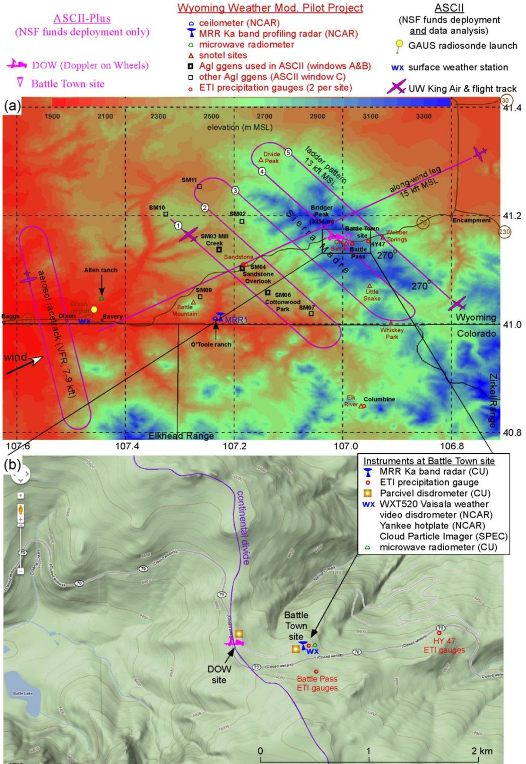
**Fig. 4:** ASCII/WWMP experimental design map, showing UWKA flight tracks and ground-based instruments. The terrain is shown in the background, in color in (a) and using contours in (b). The highways are shown as well. Panel (b) is a zoom-in of (a) around Battle Pass. The scale in (a) can be derived from the latitude/longitude values.
