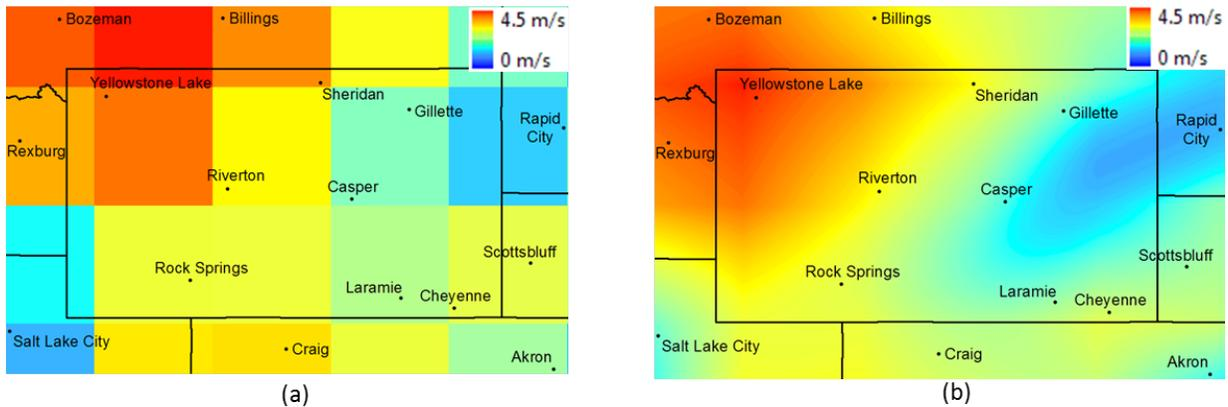
**Figure 9: Downscaling of NCEP wind speed. (a) 2 degree NCEP wind speed and (b) Spatially interpolated NCEP wind speed in 0.01 degree resolution.**
