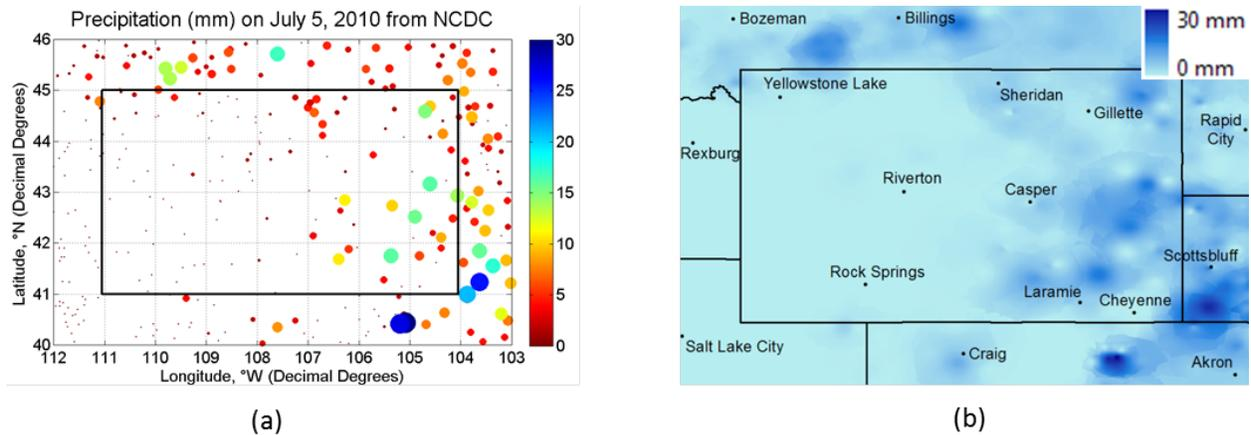
Figure 13: An example of spatial interpolation of Precipitation for July 5, 2010. (a) Observed daily precipitation at weather stations and (b) spatially interpolated precipitation.
