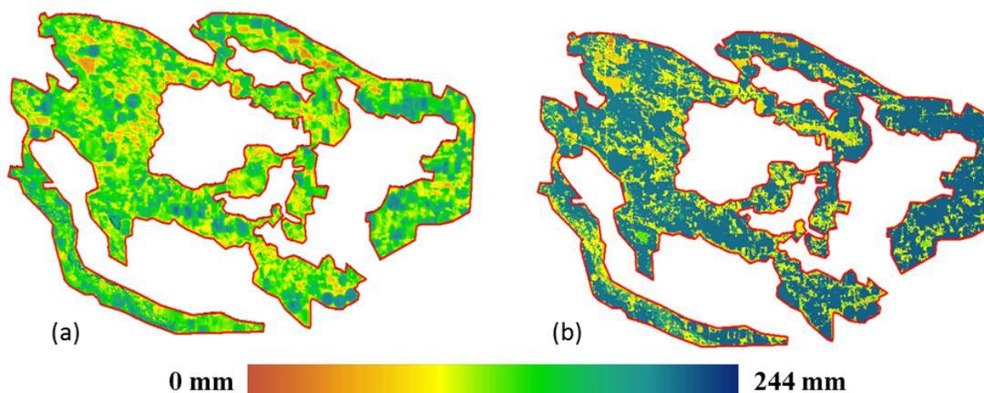
Figure 27: Spatial distribution of July 2009 ET (METRIC on the left and Wyoming ET Calculator on the right).
