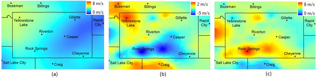
Figure 12: Final wind speed calculation: (a) NCEP - (b) wind bias = (c) final wind speed.
