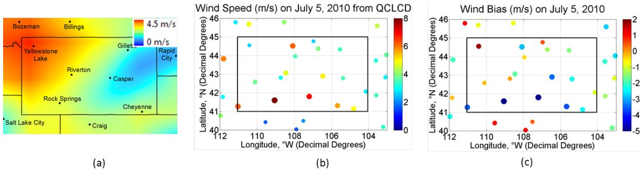
**Figure 10: Wind bias calculation: (a) NCEP wind speed – (b) observed wind speed at stations = (c) wind speed bias at stations.**
