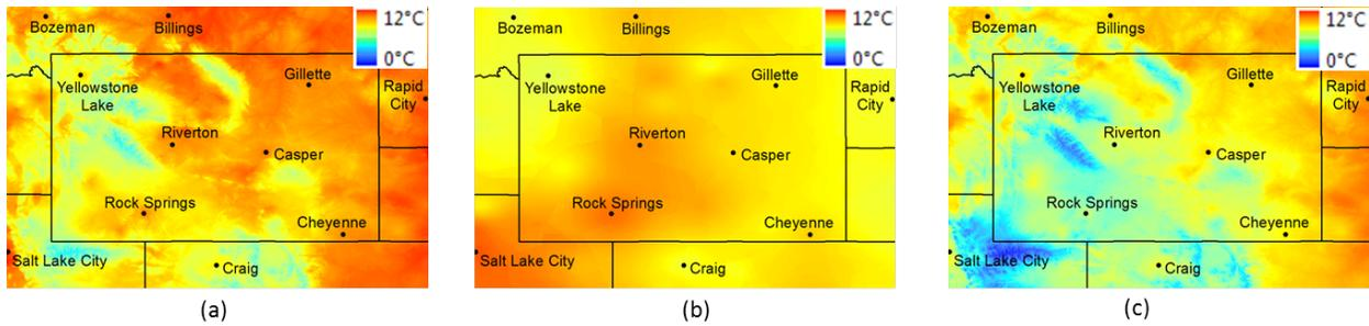
**Figure 8: Daily Dew point temperature (c) is calculated by subtracting monthly bias of the dew point temperature (b) from spatially interpolated daily dew point temperature (a).**
