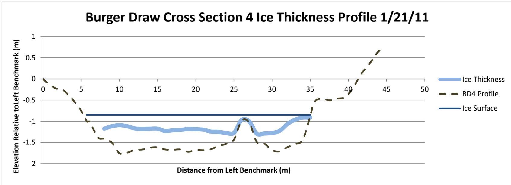
FigureA2.5: Burger Draw Cross Section 4 Ice Thickness Profile; surveyed on January 21, 2011. BD4 is upstream of Burger Draw on the Powder River, and has a continuous ice cover. The underside of the ice profile ends before the left end of the ice cover because field personnel feared driving the ice auger into the bed at that location.
