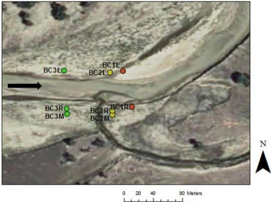
Figure A1.1. Aerial image of the Beaver Creek—Powder River confluence showing the relative positions of the cross sections in the Powder River. Cross sections BC1 and BC2 are downstream of Beaver Creek while BC3 is upstream Beaver Creek. The arrow indicates flow direction of the Powder River. Distances (upstream or downstream) of the cross sections from the tributary confluence are: BC1: 30m, BC2: 10m, BC3: 40m.
