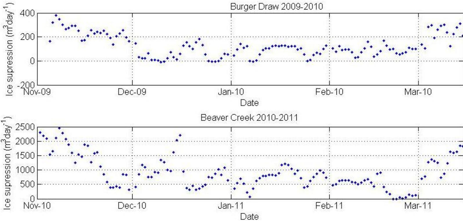
Figure 3.12. Daily ice suppression in Powder River caused by CBM product water heat delivered by Burger Draw (top) and Beaver Creek (bottom). The maximum ice suppression at Burger Draw was  $380\text{m}^3\text{day}^{-1}$ , while Beaver Creek has a maximum ice suppression of  $2450\text{m}^3\text{day}^{-1}$ . The large, almost continuous heat flux supplied by these drainages maintained open water leads downstream of confluences throughout the two winters of the study
