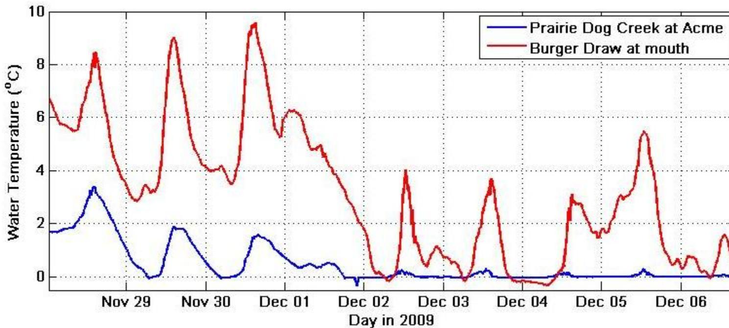
Figure 3.1. Plot of water temperatures in *Prairie Dog Creek at Acme* and *Burger Draw at mouth* during freeze-up in 2009. The *Prairie Dog Creek* temperature record is typical for the freeze up period for many small Wyoming streams. By contrast, the effect of warm CBM product water discharge into *Burger Draw* is indicated by the elevated temperatures in the temperature record for this stream.
