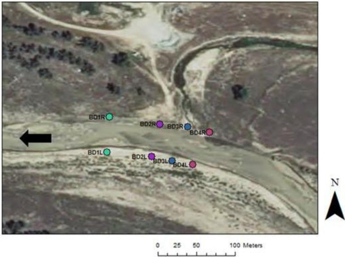
Figure A1.2. Aerial image of the Burger Draw—Powder River confluence showing the relative positions of the cross sections in the Powder River. Cross sections BD1, BD2, and BD3 are downstream of Burger Draw while BD4 is upstream. The arrow indicates flow direction of the Powder River. Distances (upstream or downstream) of the cross sections from the tributary confluence are: BD1: 80m, BD2: 30m, BD3: 5m, BD4: 15m
