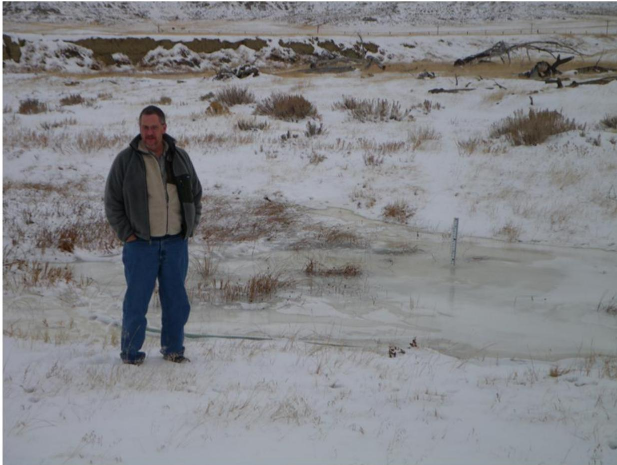
Figure 3.6. The staff gage at *Burger Draw at mouth*, a water temperature logging station located 50 m from the mouth of Burger Draw. The ice accumulation (aufeis) shown here is exceeds 30cm in thickness, and extends outside the natural channel boundaries.
