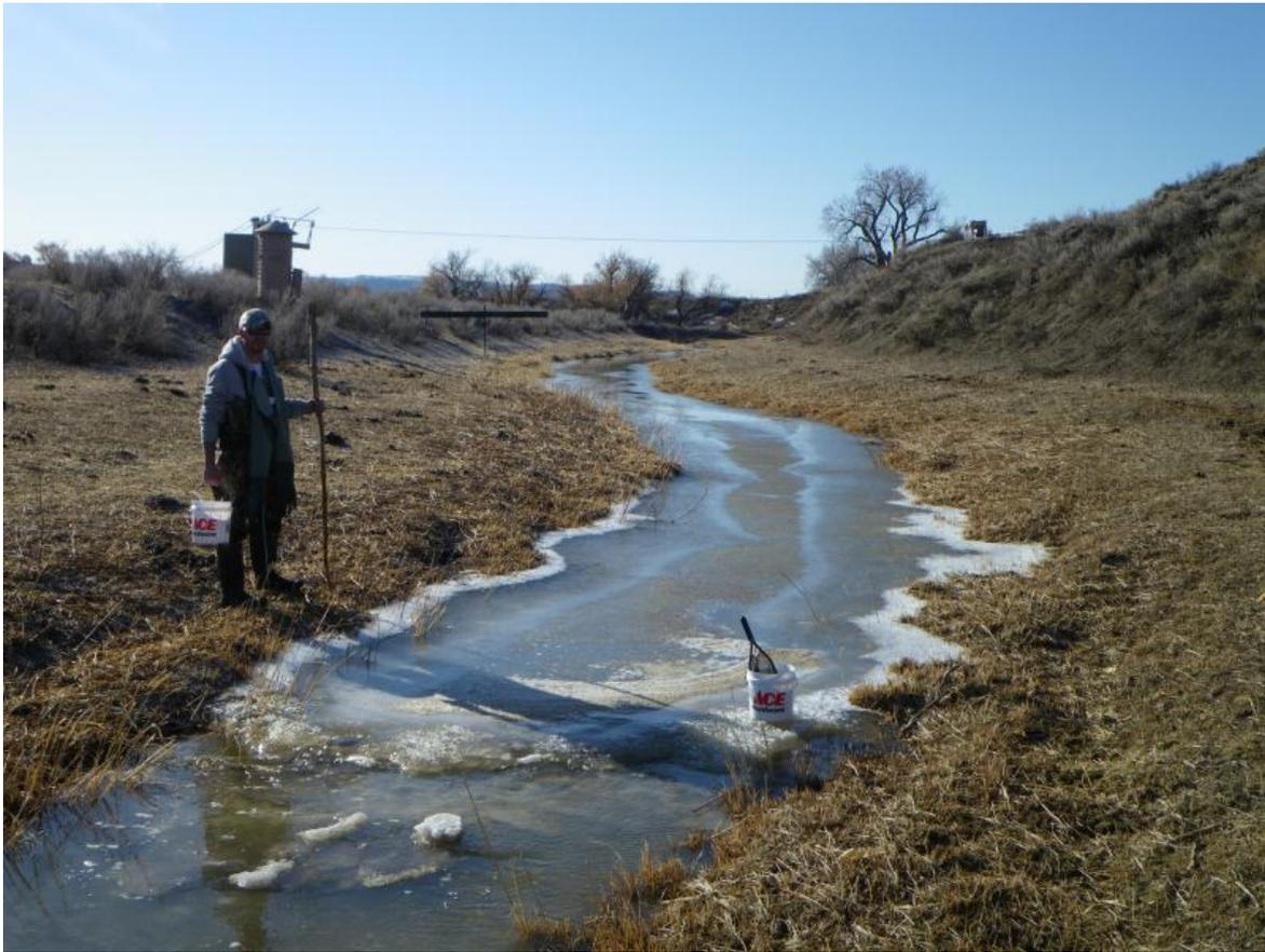
Figure 3.3. An anchor ice dam on Prairie Dog Creek, March 4, 2010. The vertical culvert pipe and cableway about 50 m in the background mark the position of the USGS gaging station, Prairie Dog Creek Acme (06306250). The anchor ice dam formed at night and was in place long enough for a thin layer of border ice to form on the backwater created by the dam.
