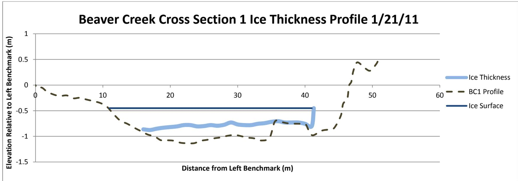
FigureA2.1: Beaver Creek Cross Section 1 Ice Thickness Profile, surveyed on January 21, 2011. BC1 has an open water lead on the right end of the profile that is roughly 5 meters wide. The Ice thickness is continuous throughout the profile till the open water lead. BD1 is 25 meters downstream of the mouth of Beaver Creek.
