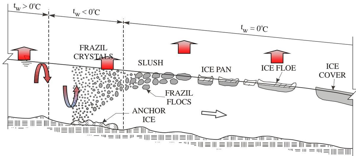
Figure 1.1 Sketch showing longitudinal river profile during ice formation. In turbulent river flow, the water becomes supercooled through heat loss to the atmosphere (red arrows); as a result the first ice to form is frazil and anchor ice. This frazil and anchor ice eventually rises to the surface and is incorporated into the growing thermal ice cover (right side of figure).
