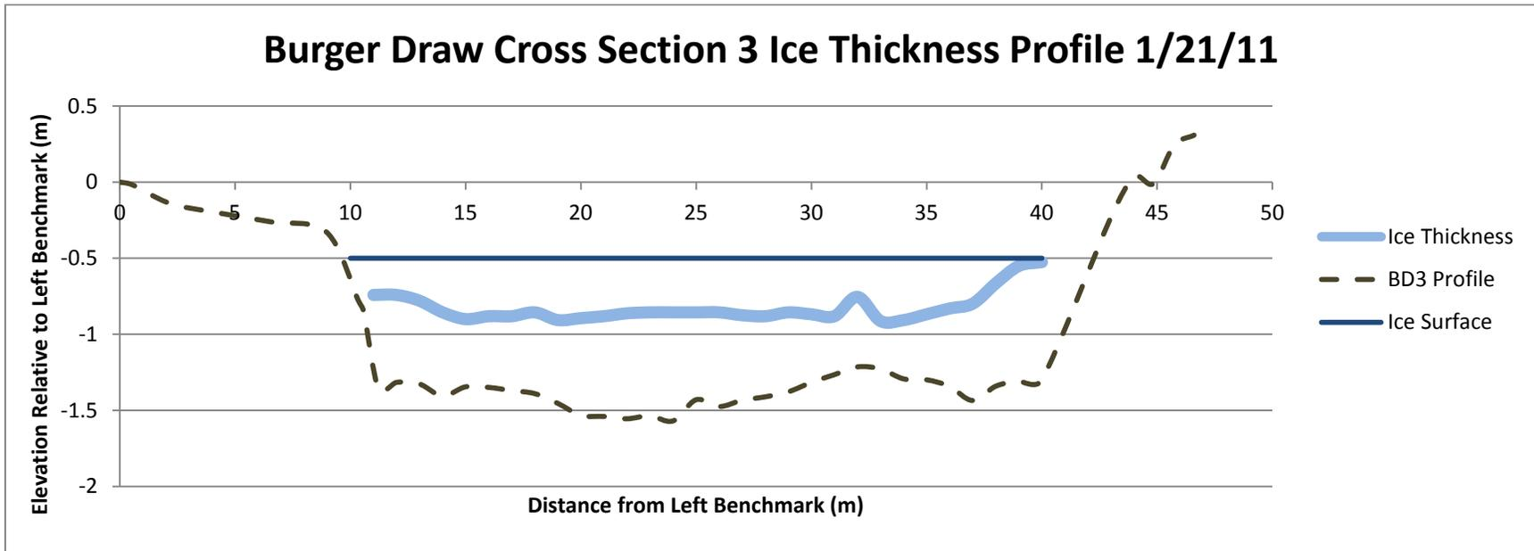
Figure A2.4: Burger Draw Cross Section 3 Ice Thickness Profile, surveyed on January 21, 2011. BD3 is the cross section closest to the mouth of Burger Draw and is directly downstream of the confluence. A small open water lead formed on the right side of the river. The ice thickness is fairly consistent throughout the profile till it draws near the open water lead end and thins rapidly.
