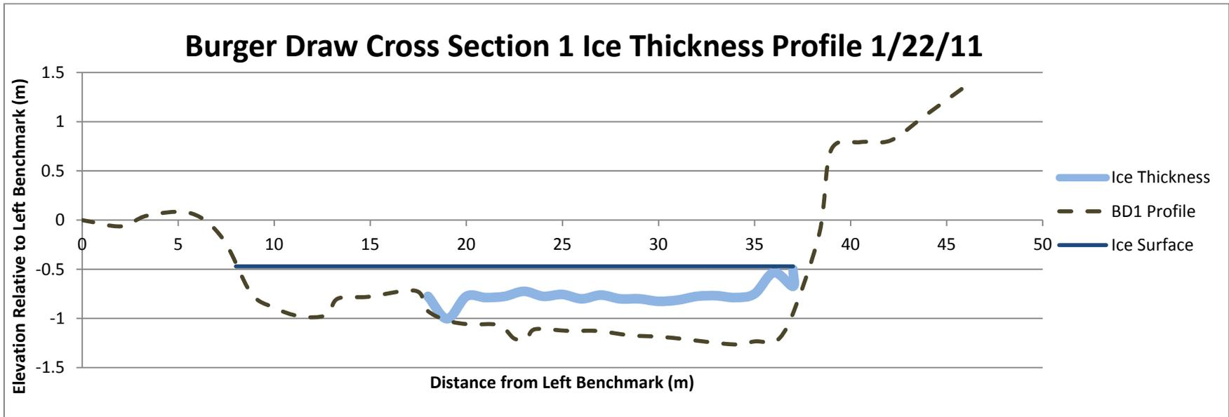
Figure A2.3. Burger Draw Cross Section 1 Ice Thickness Profile was surveyed on January 21, 2011. BD1 has a 1 meter wide open water lead on the right end of the profile. BD1 is 80 meters downstream the mouth of Burger Draw. Ice froze to the bed from left water edge to about 17 meters from the left benchmark.
