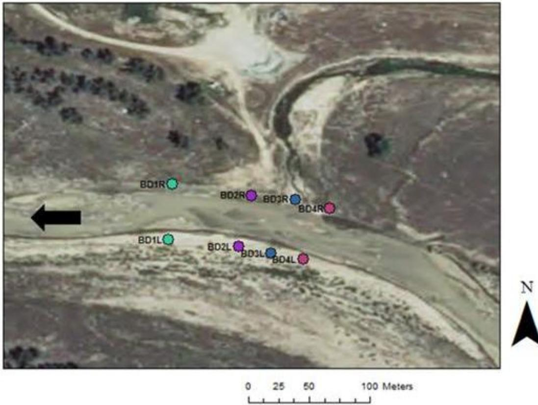
Figure 2.3. Aerial image of the Burger Draw—Powder River confluence showing the relative positions of the Burger Draw cross sections. Cross sections BD1, BD2, and BD3 are downstream of Burger Draw while BD4 is upstream. The arrow indicates flow direction of the Powder River. Distances (upstream or downstream) of the cross sections from the tributary confluence are: BD1: 80m, BD2: 30m, BD3: 5m, BD4: 15m.
