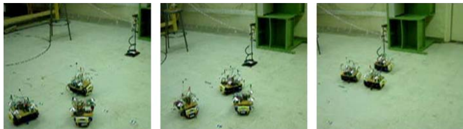
Figure 2. A laboratory-scale CPT scenario, in which miniature robotic vehicles successfully find a source of ethanol vapor (top-right)
