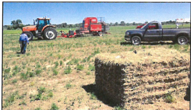
A machine featured at the forage day picks up smaller bales and combines them into one.
