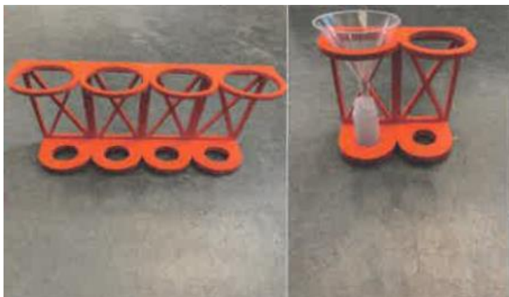
Figure: 3D printed sample of the filtration rack.
