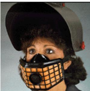
APRs equipped with particulate filters capture particles (dusts, mists, fumes) before they reach the user’s breathing zone. These respirators do not protect against gases or vapors. Filters should be replaced when user finds it difficult to breathe through them or the user can sense the surrounding contaminated environment. These devices cannot be used in atmospheres considered IDLH. You must be enrolled in the UW Respiratory Protection Program to use this type of respirator.
