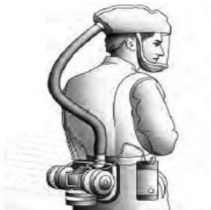
A PAPR has a blower that pulls air through attached filters. The blower then pushes the filtered air into the face piece, which covers the user's face. For loose-fitting PAPRs, fit testing is not required and these units can be used by workers with facial hair. Tight fitting PAPRs must be fit tested. These devices cannot be used in atmospheres considered IDLH. You must be enrolled in the UW Respiratory Protection Program to use this type of respirator.
