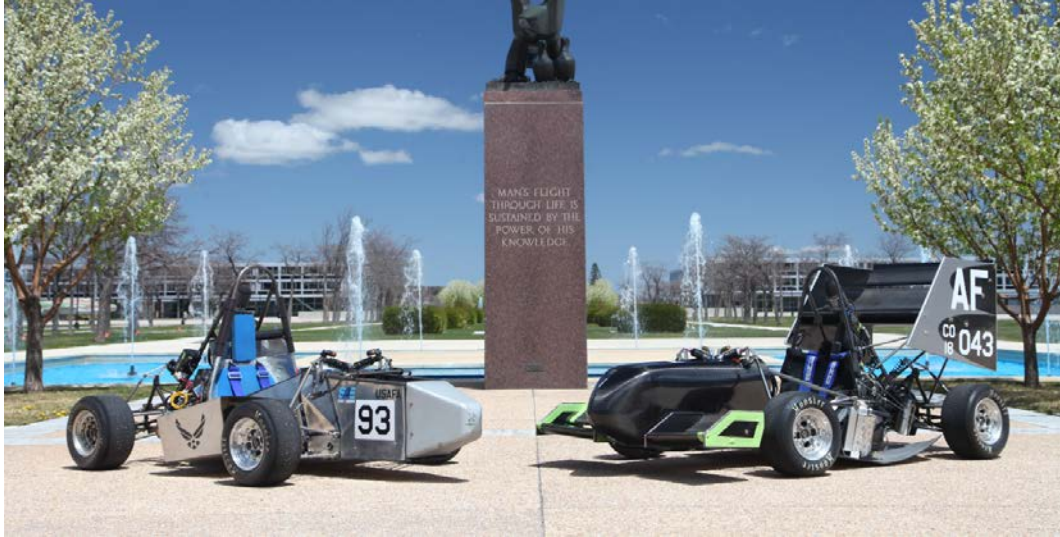
Figure 1: U.S. Air Force Academy Formula SAE vehicles from 2017 (left) and 2018 (right). The 2017 competition was only the second time since 1999 that the team completed all the competition events. Aerodynamic downforce wings were first incorporated in 2018.
