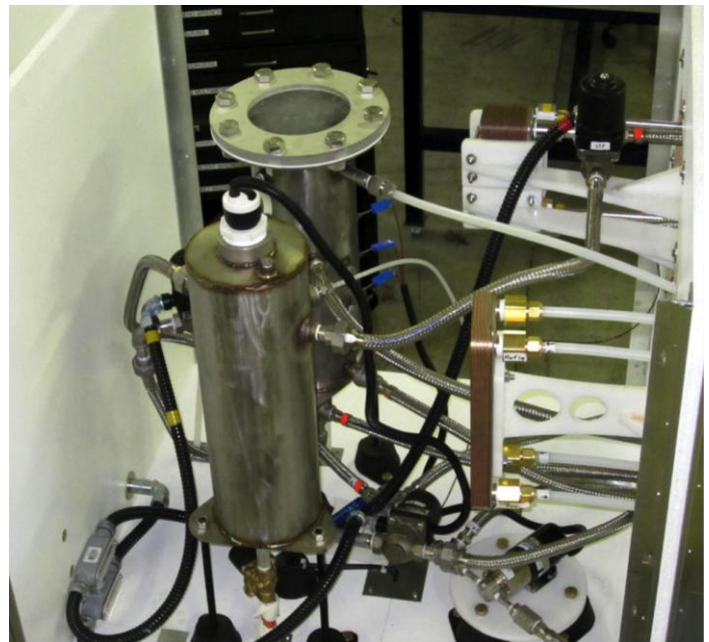
Primary coldbox containing (clockwise, from top left) the desublimating heat exchanger, liquid cooler, gas recuperator, contact liquid pump, and contact liquid reservoir.
