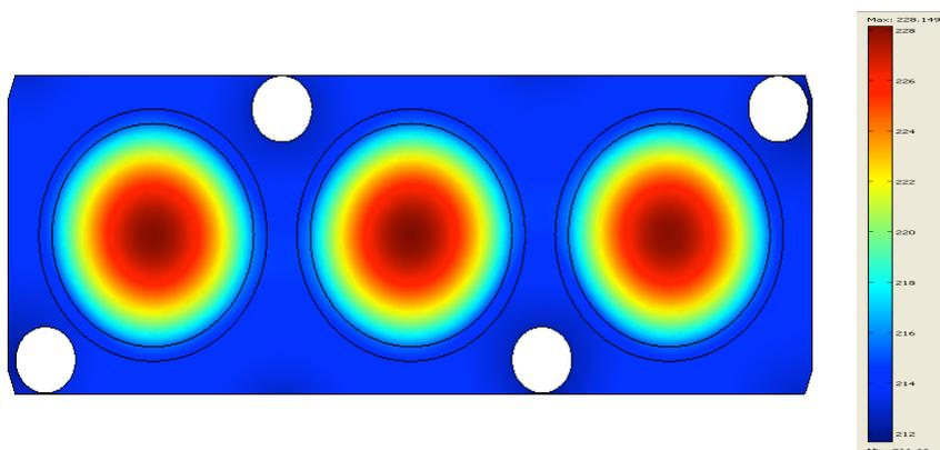
Figure 10. Temperature profile ( $^{\circ}$  C) of the configuration of 4 cooling tubes
