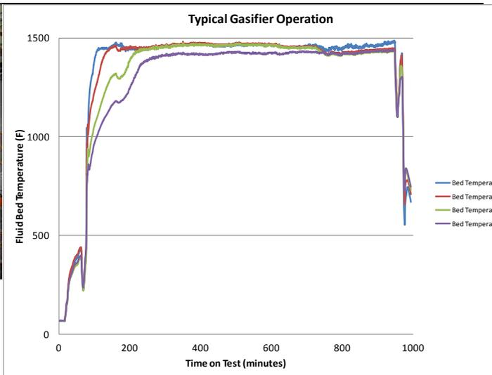
Figure 12. Typical Gasifier Bed Temperatures
