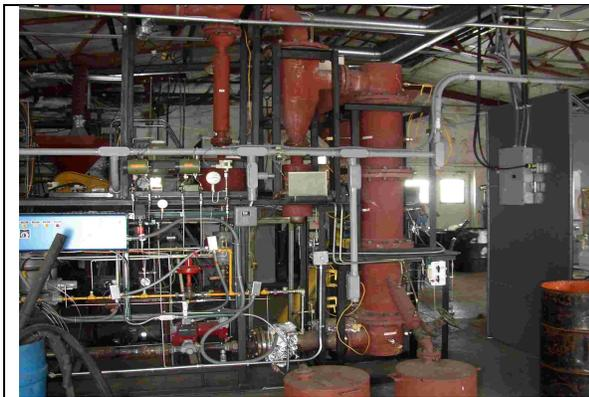
Figure 11. WRI Fluidized-Bed Gasifier
