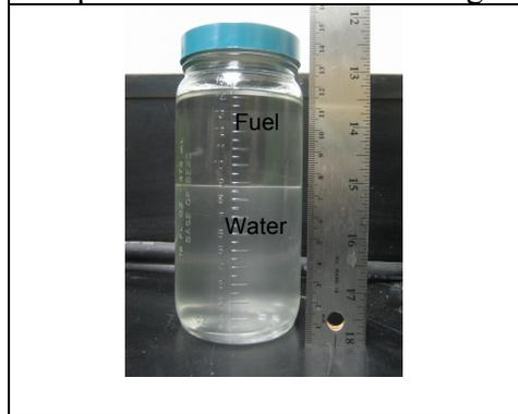
Figure 2. Liquid hydrocarbon product yielded from FT reactor (235 °C)
