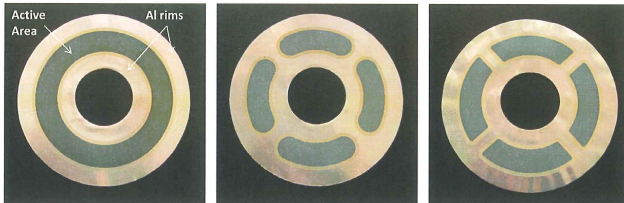
Figure 1. Donut shaped membranes of alternate design for thermal expansion issues
