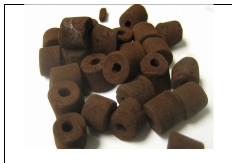
Figure 1. FeCuK FT catalyst on La promoted 8 mm alumina rings
