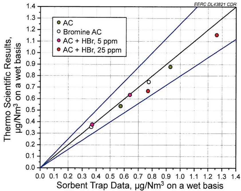
Figure ES-6. Summary of Thermo Scientific CMM results when Wyoming PRB coal with bromine addition was fired.
