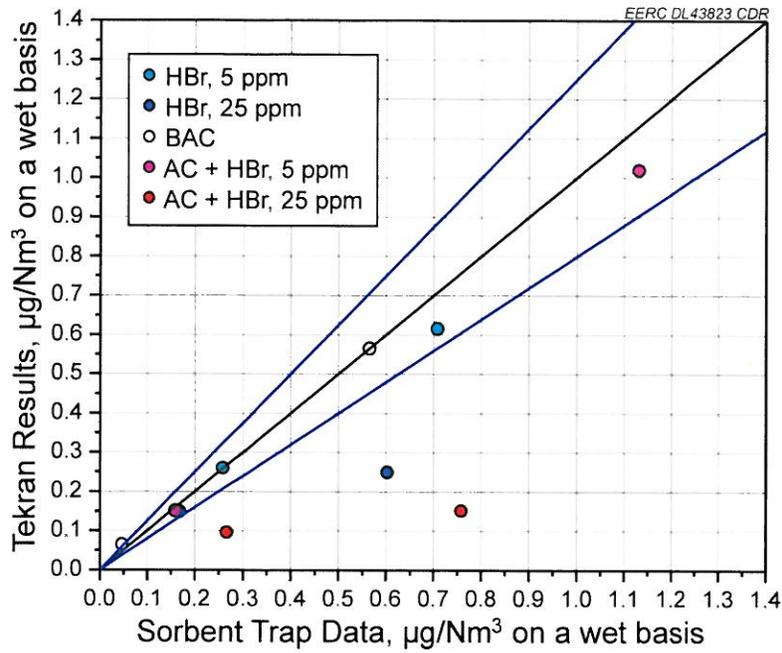
Figure ES-3. Summary of Tekran CMM results when natural gas with bromine addition was fired.
