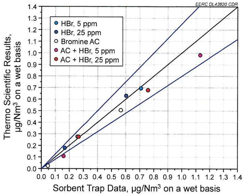
Figure ES-5. Summary of Thermo Scientific CMM when natural gas with bromine addition was fired.
