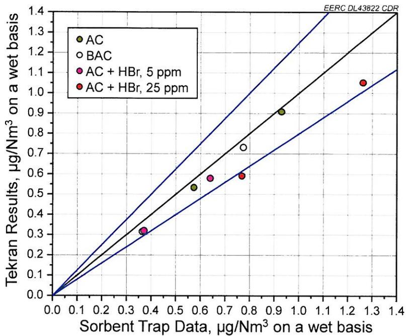
Figure ES-4. Summary Tekran CMM results when Wyoming PRB coal with bromine addition was fired.
