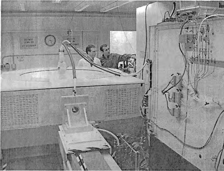
Encana Three-Phase Flow Laboratory in action. Graduate student Morteza Akbarabadi and Dr. Mohammad Piri discuss flow experiments with supercritical CO 2 . A CT scanner is at the horizontal orientation with a heated core-holder held by a vertical positioning system in the middle. The scanner is used to characterize three-phase flow in rock cores at reservoir conditions.
