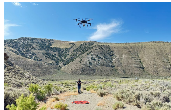
Pictured: Kyle Summerfield, program manager of the 3D Visualization Center, or Viz Center, within the University of Wyoming's School of Energy Resources, operates the HySpex Mjolnir VS-620 mounted on a heavy-lift drone in southwest Wyoming.
